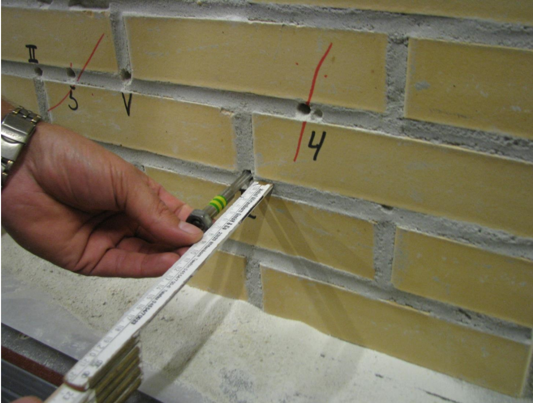
Figure 4. Determining the distance L_i . The distance is measured before and after the X-drill has been knocked in.
