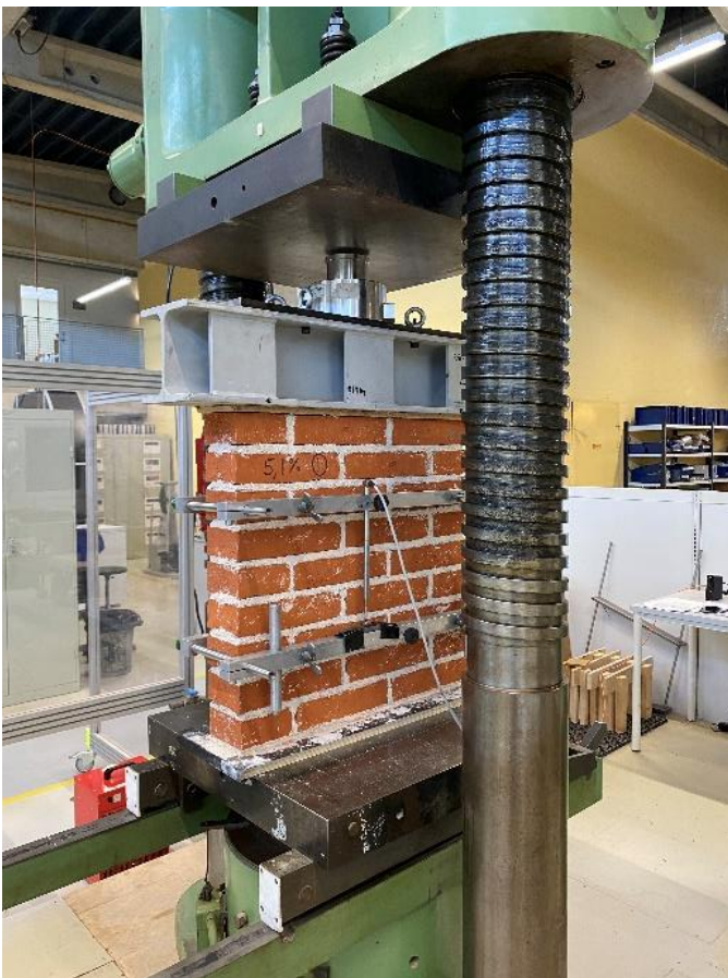
Photo 1: Test of wall specimens. Axial deformations were recorded on front and back of the wall along with the applied load.
