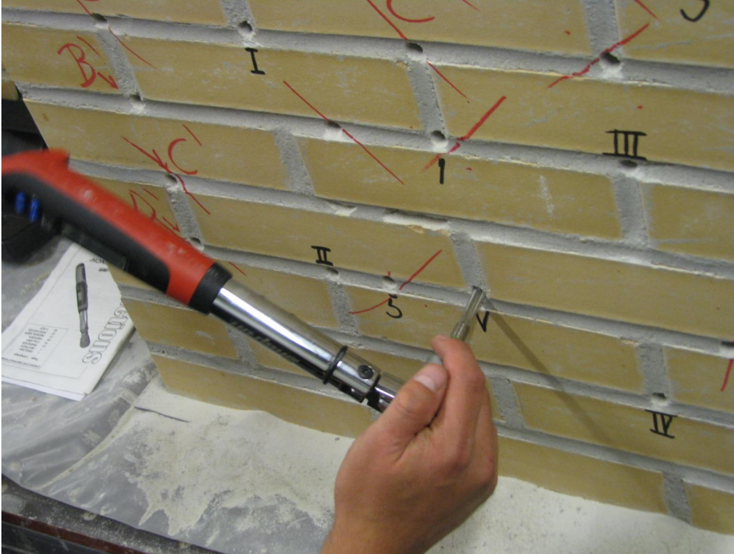
Figure 6. Torque wrench is used to determine M_v . The torque wrench is turned slowly with one hand at the same time the X-drill is held with the other hand so that the effect of force is as much as possible a pure twisting torque.
