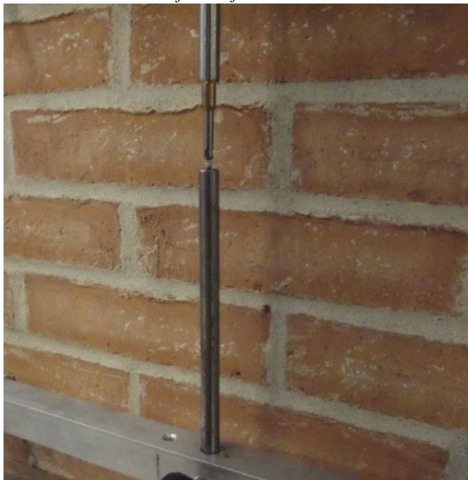
Picture 2: Placement of the deformation transducer on the steel rod.
