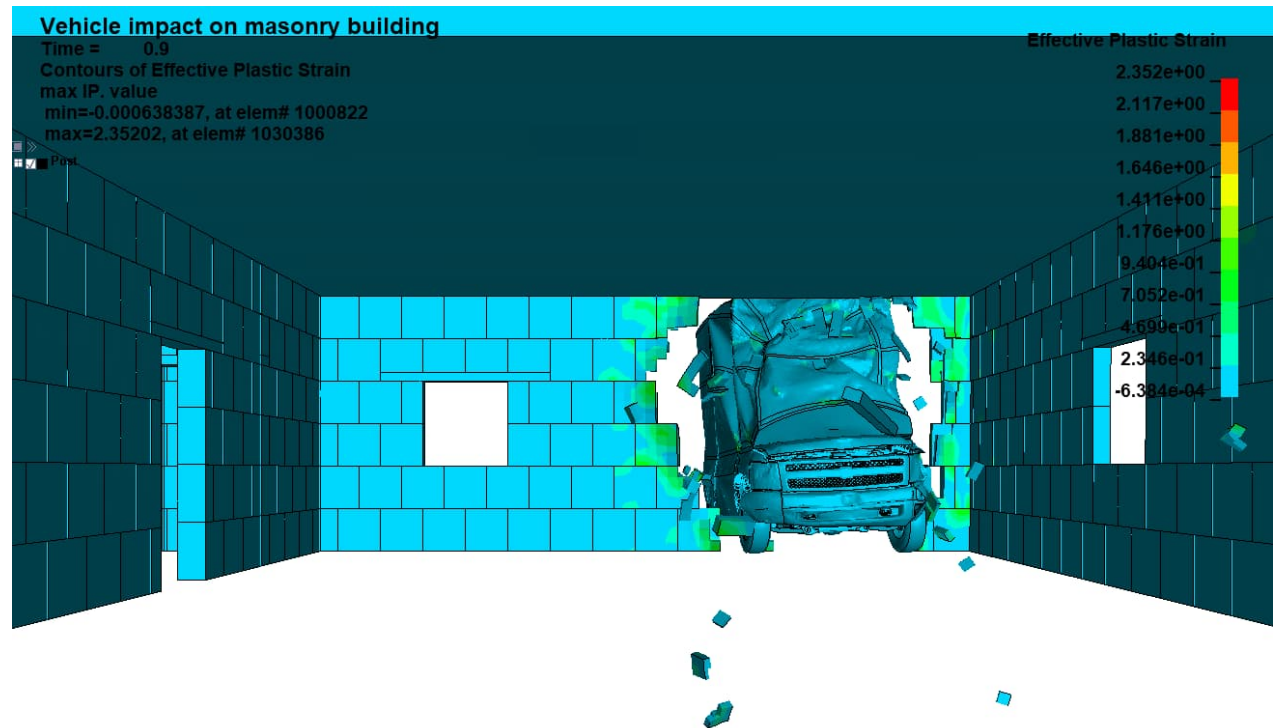
Figure 26. Close-up views of the impact mechanism from the exterior and interior of the building, highlighting the damage caused by the impact in the form of fragments and effective plastic strains.
