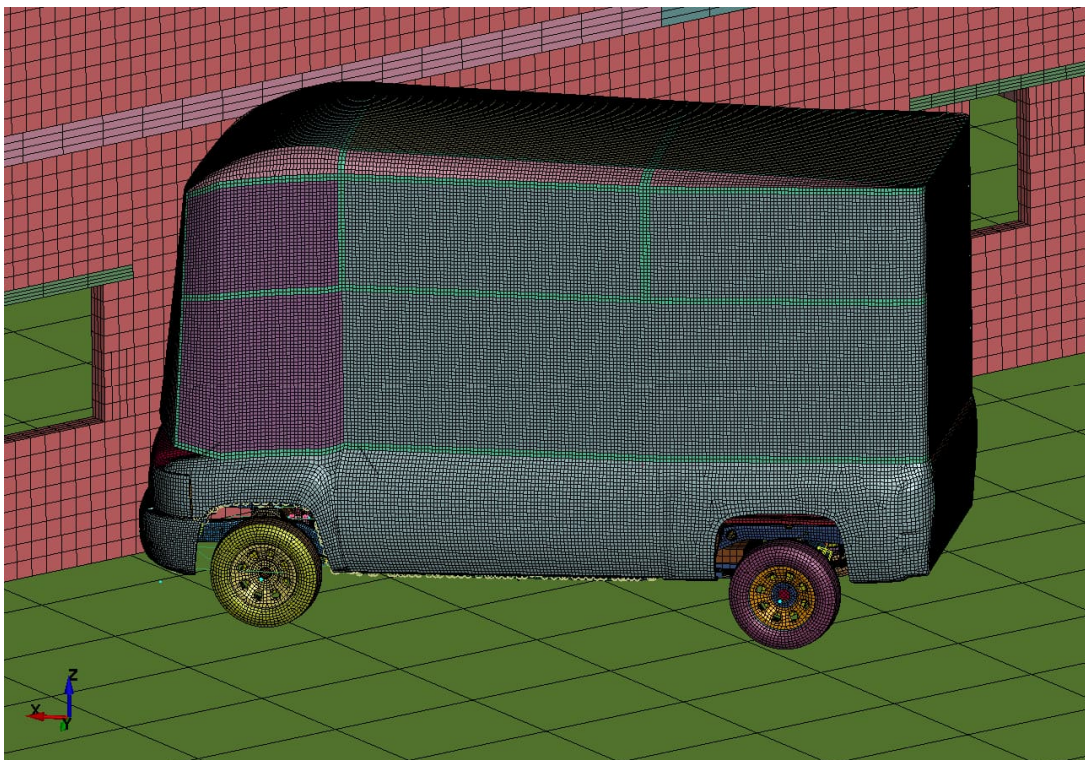
Figure 17. The Finite element model of the vehicle, composed primarily of shell finite elements.
