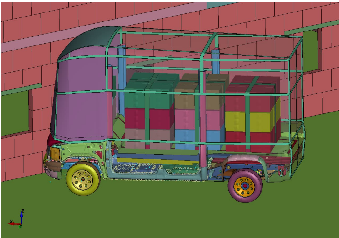
Figure 16. The 2019 Generic Large-size (Automated Driving System ADS) Vehicle Model used in the simulation, as provided by the Center for Collision Safety and Analysis (CCSA) at George Mason University.
