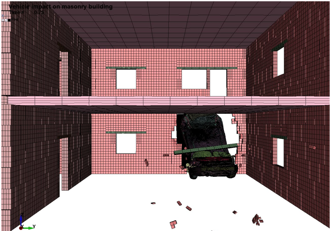
Figure 34. Close-up views of the impact mechanism from the exterior and interior of the building, showing the damage state of the finite element model after 0.75 s.
