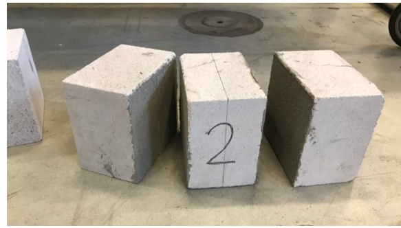
Figure 77: Failure type of sample 2
