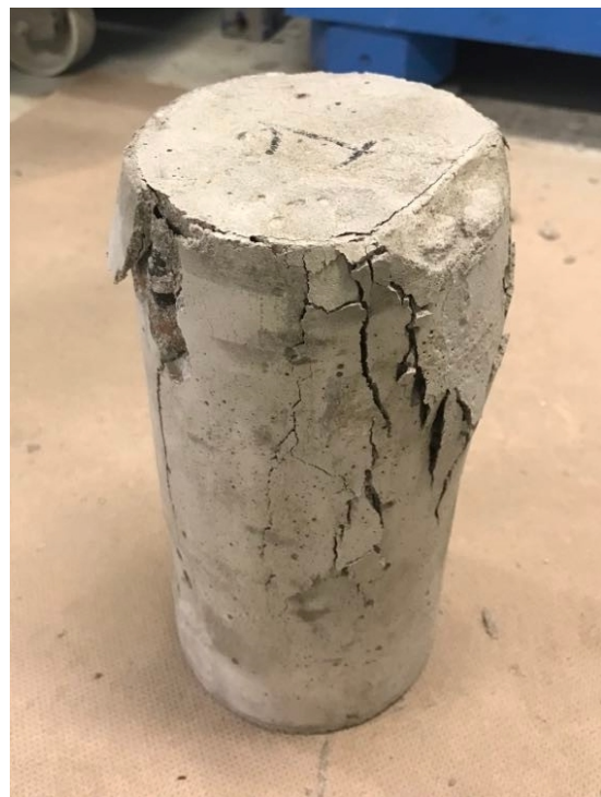
Figure 40: Failure of cylinder 1
