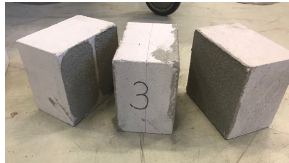
Figure 79: Failure type of sample 3
