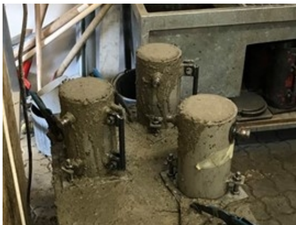
Figure 66: Concrete filled cylinder molds
