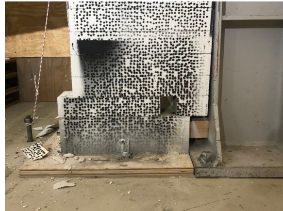
(f) Foundation failure right pillar
