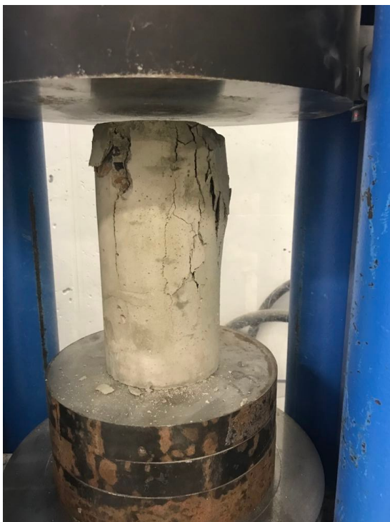
Figure 39: Concrete cylinder test setup
