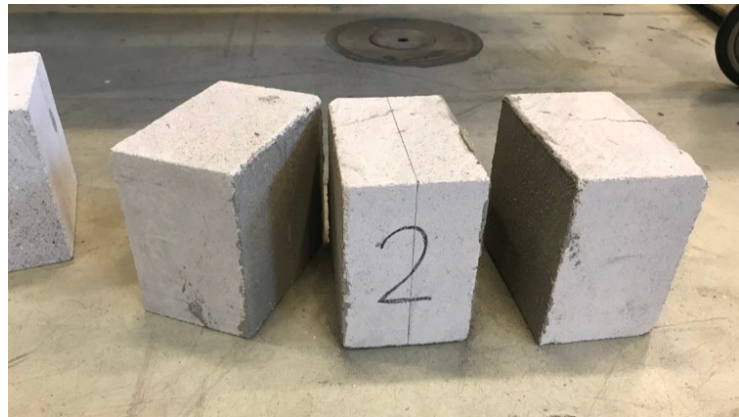
Figure 42: Failure in mortar sample 2
